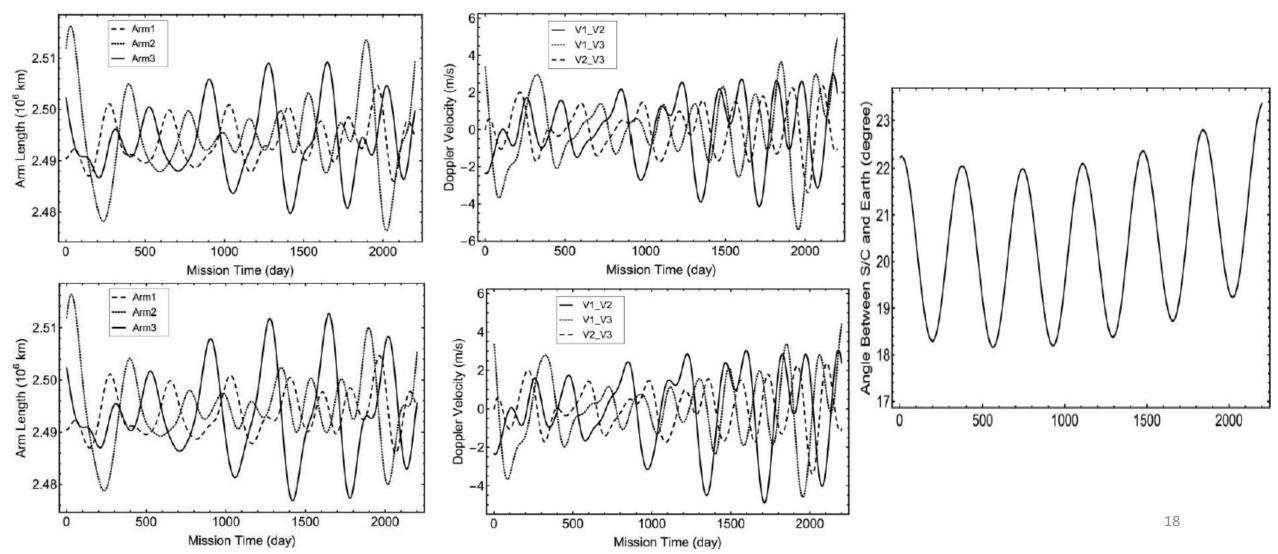
Variations of the arm lengths and the velocities in the line of sight direction in 2200 days for the TAIJI S/C configuration with initial condition adjustment
